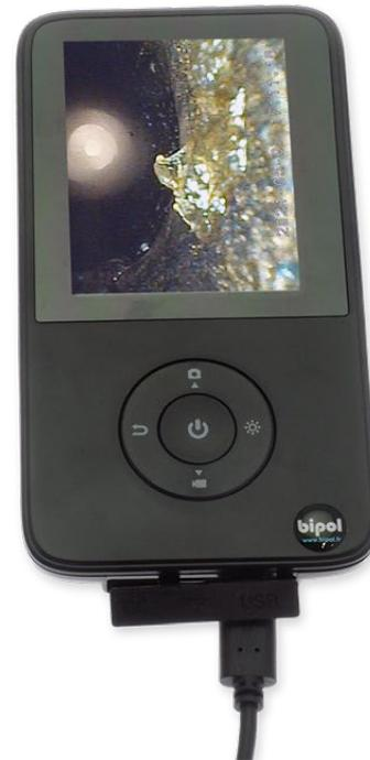
Quick inspection of any bore from 2.2 mm.
